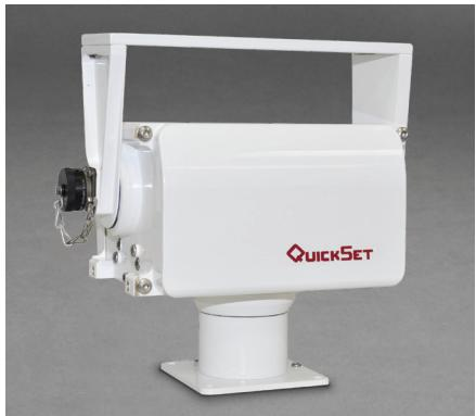
The QPT-20 Series of pan & tilt positioners is designed for a wide variety of sensor position applications. The QPT-20 Series is rugged and durable enough for virtually any environment, including port surveillance and mobile vehicle vision systems. Stepper motor models can handle up to 20 lb-ft. of torque for heavier payloads. The brush motor QPT-20 models can handle payloads up to 8 lb-ft. Both provide
