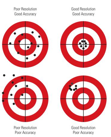
Resolution refers to how small an angle the pan/tilt can be commanded to, or how small an angle the position can be reported. Accuracy refers to how close the commanded position is to the desired position.
