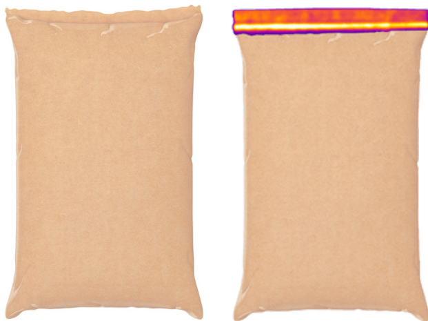
Visible and IR images of a plastic bag demonstrating opacity in the visible spectrum and transparency in the infrared wavebands.
