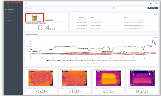
A customizable comprehensive dashboard display highlights sensor measurements, camera imagery, sensor health, and alarm status.
