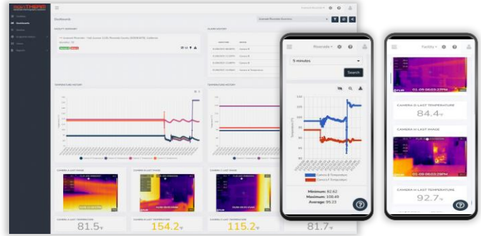
A customizable comprehensive dashboard display highlights sensor measurements, camera imagery, sensor health, and alarm status.
