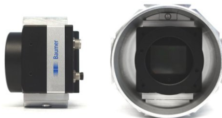
The mount guarantees excellent heat dissipation
