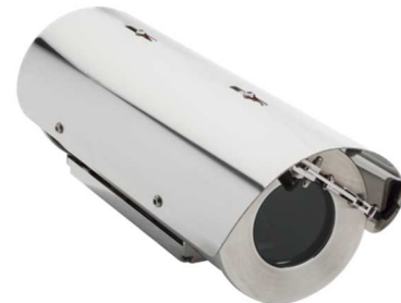
129WW CAMERA HOUSING WITH SUNSHIELD, HEATER AND WIPER
