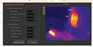
Emissivity correction enables you to match the emissivity characteristics of different target materials in your inspection image. Temperature readings are reliable for homogenous objects made of a single material, or objects composed of several different source materials.
