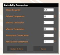
The software includes several unique. advanced features for research and development tasks. For examthe advanced ple, global and regional emissivity correction functions enable you to optimize the accuracy of your temperature
