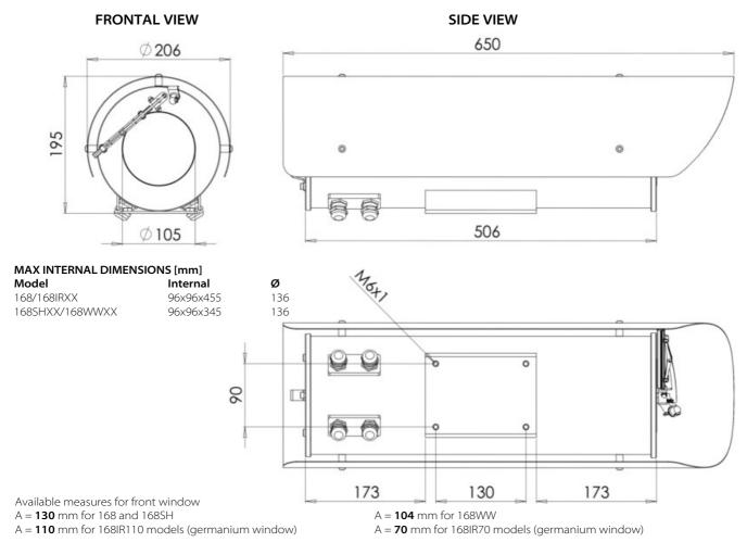
$Dimensions\ in\ millimetres-Tolerances\ according\ QMS-Design\ and\ product\ specifications\ subject\ to\ change\ without\ notice$
