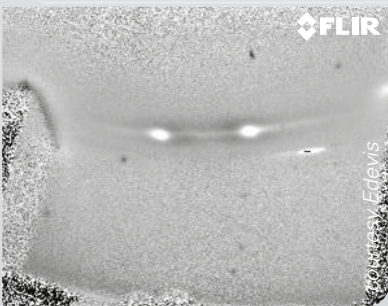
Inductive crack detection
