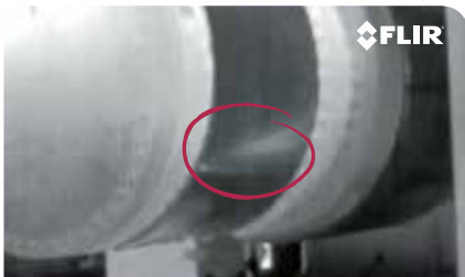
Captured gas leak from production site.
