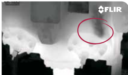
Captured gas leak.
