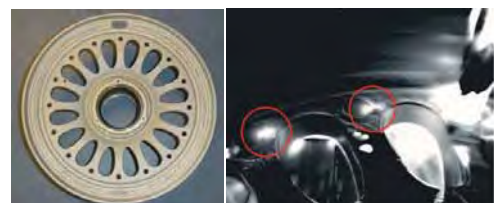
Aluminum aircraft wheel with cracks detected.
